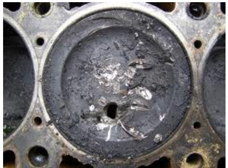
A piston top with a hole in it and other damage that resulted from a broken timing belt.
