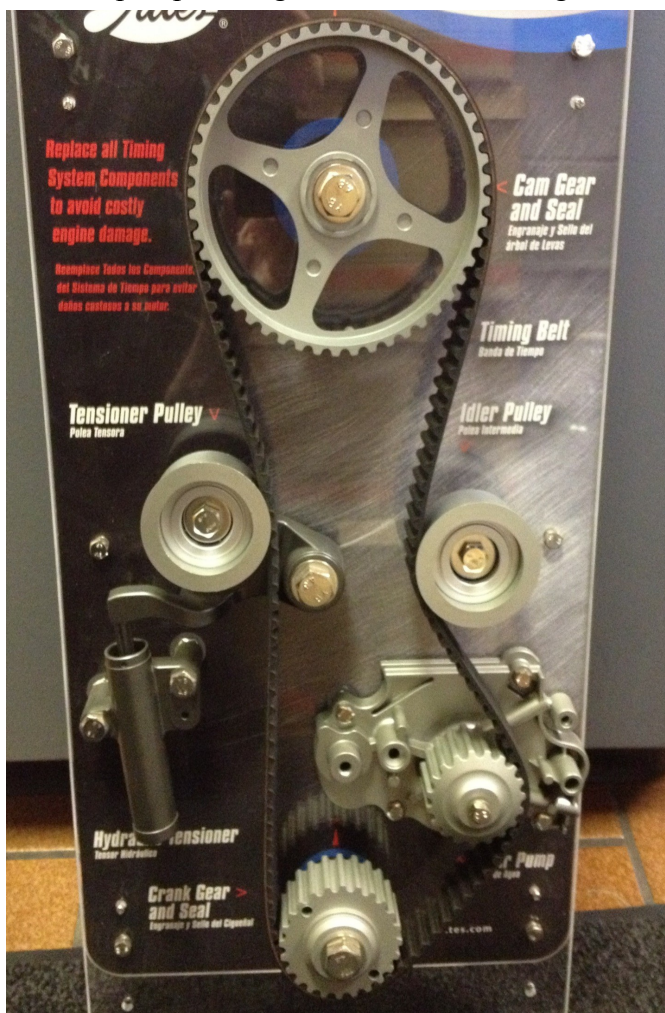
This is a timing belt display that features a typical four cylinder timing belt and components.
