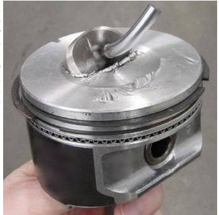
A broken valve that stuck in a piston when a timing belt broke.
